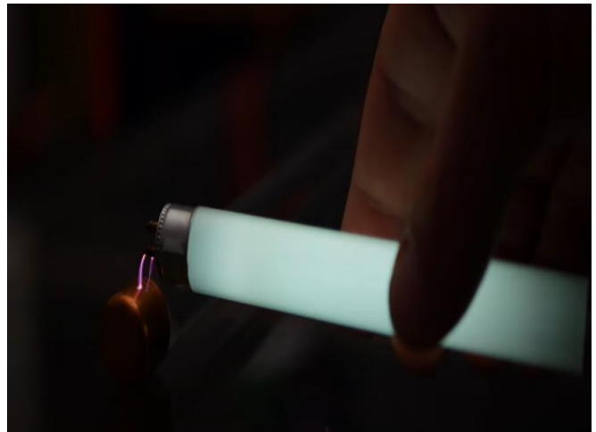
Fig. 5: After turning ON the supply from the Tesla coil we can see that the CFL tube placed beside the Copper capping starts conducting wirelessly.
