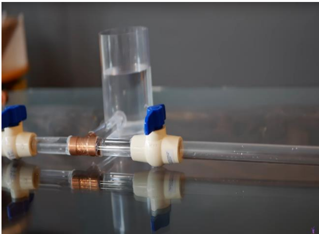
Fig. 1: Experimental setup of conduction of electricity through pipes containing salt water.
