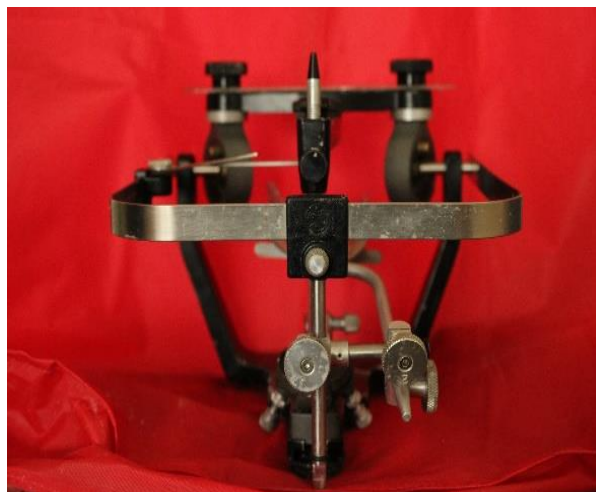
Fig. 17: Facebow Transfer Hanau Wide Vu Semi Adjustable Articulator
