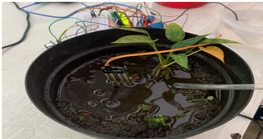
Fig. 4(b): Soil moisture is wet and water irrigation pump OFF
