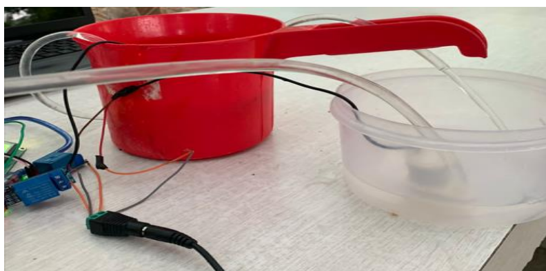
Fig. 4(c): Water level is low and water tank pump ON
