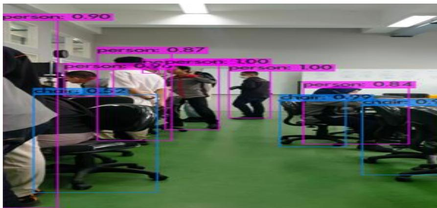
Fig. 4: YOLO-v3 performance in detecting three different types of things
