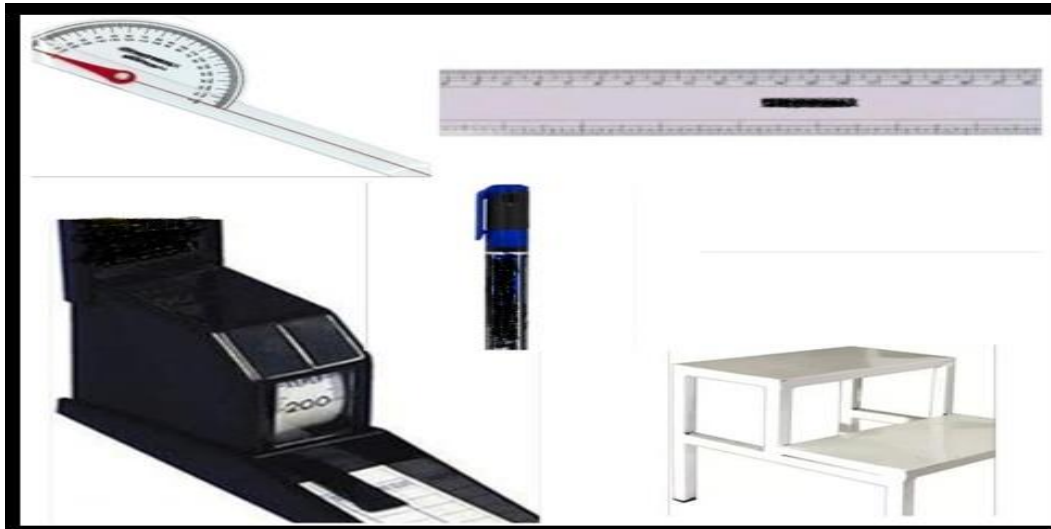
Fig. 1: Universal goniometer, Ruler, Stadiometer, Marker, Steel Platform
