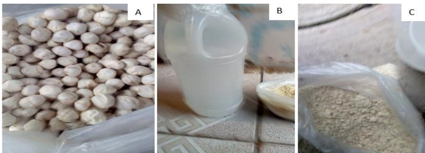
Plate 1 Preparation of Bio-Sorbent; A (Peeled Moringa Seed); B (Floating Liquid); and C (Crushed Moringa Seed)
