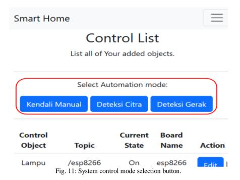
There is a selection of control modes, namely manual mode, namely controlling lighting conventionally, image sensor mode, namely automatic control of lights based on the number of human objects captured by the sensor in the room. Motion sensor mode is light control based on the presence of objects in the room. Modes can be selected and adjusted to suit your needs.
