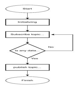
Fig. 4: Data flow diagram for broker node
