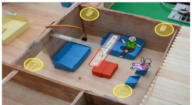
Fig. 17: Red line (automatically controlled lights) and yellow line (manually controlled).
