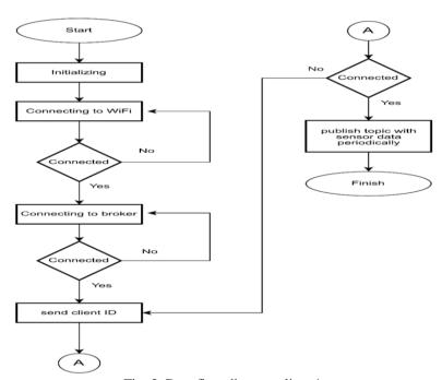
Fig. 3: Data flow diagram client 1
