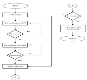
Fig. 5: Data flow diagram for lights node.
