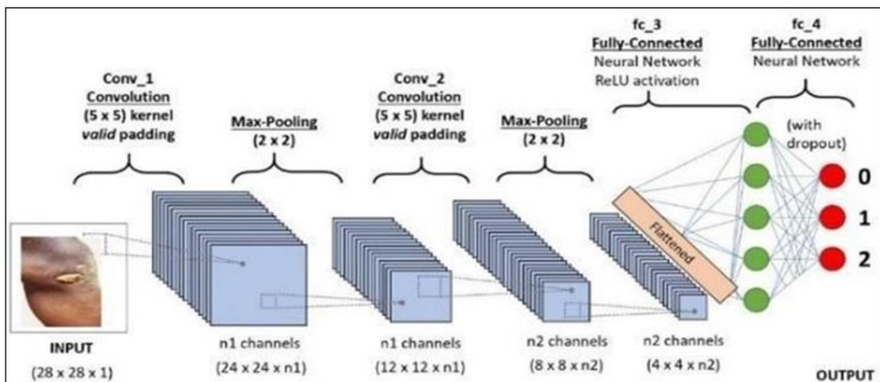
Fig 2 Proposed CNN Operation
