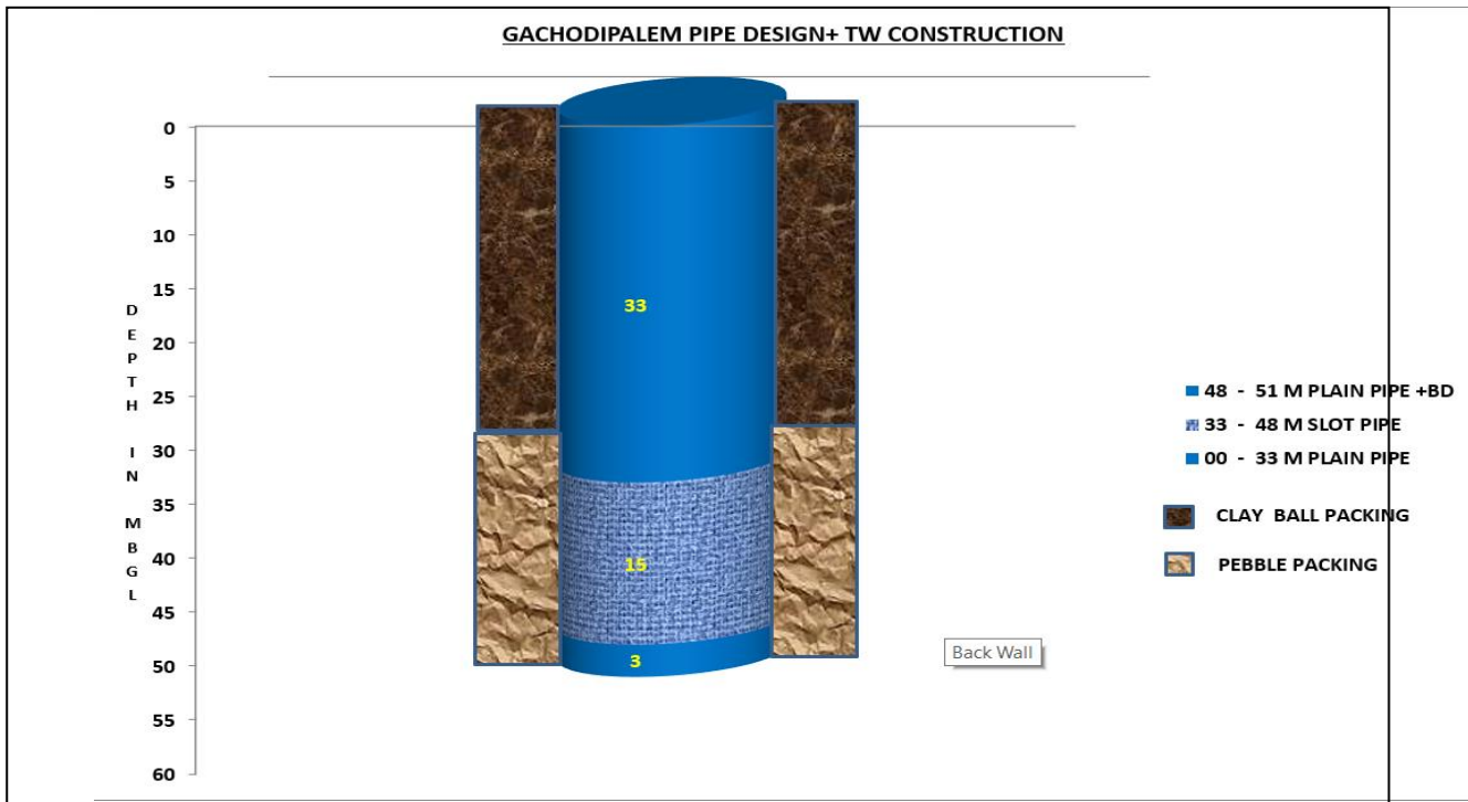
Fig. 5: Pipe design & tube well construction
