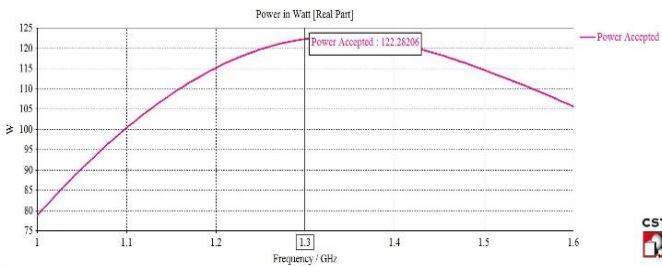
Fig. 20:- Array accepted power.
