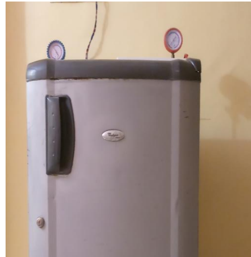
Fig. 2: Domestic Refrigerator with pressure gauges
