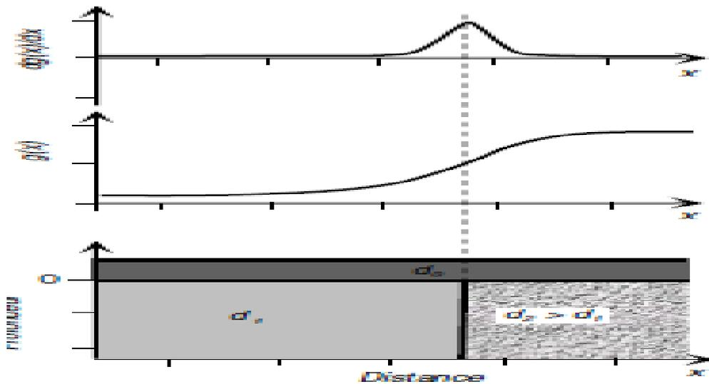
Fig. 5: Difference between the curves of the horizontal gradient and the Bouguer anomaly above a contact (Jacques Dubois, 2011 [6]).
