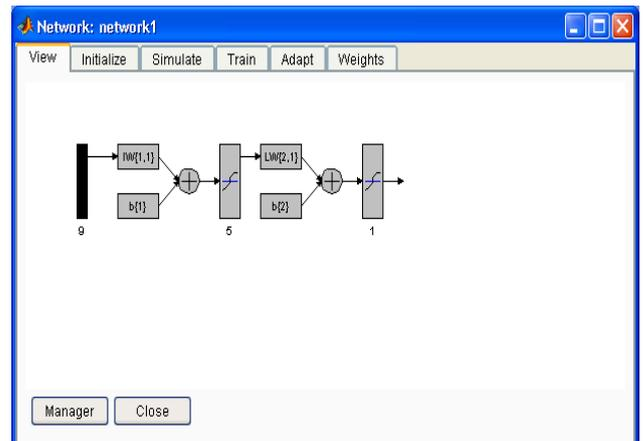
Fig. 11: Architecture of neural network
