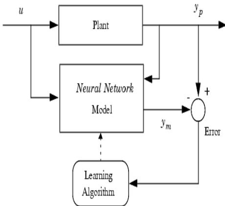
Fig. 1: Plant model used by the controller to predict future performance
