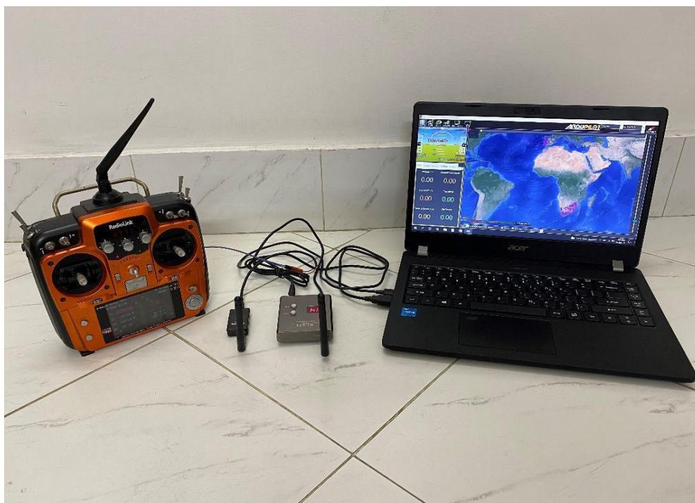
Fig. 30: Prototype of the ground station
