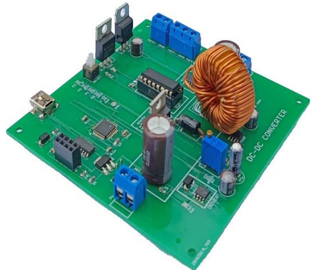
Fig. 5: A fabricated DC-DC Converter with PI Controller.
