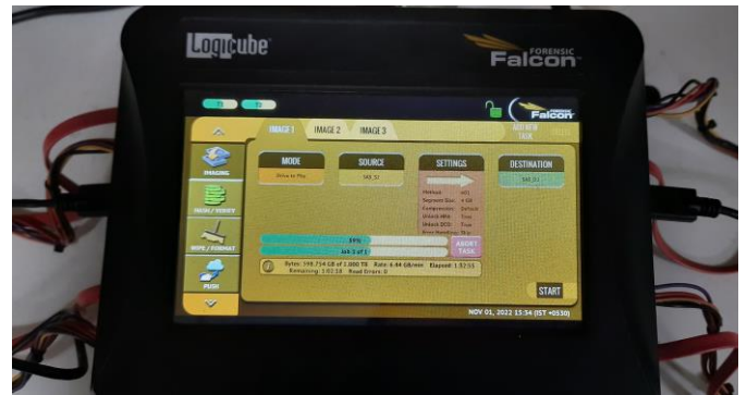
Fig 1:- FALCON Imager used for preparing bit stream image of infected hard disk
