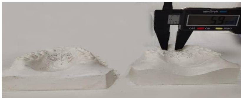
Fig. 2: Dental cast analysis using digital verniercaliper
