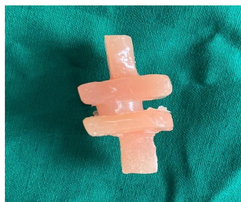
Fig. 1: Acrylic specimen with the acrylic based denture liner injected in between
