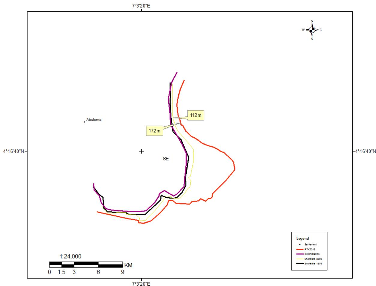
Fig 8: Overlay of 1986 shoreline, 2000, 2013 and RTK at Abuloma axis
