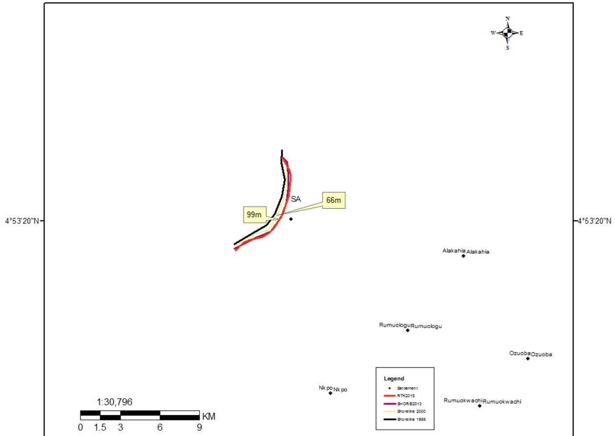
Fig 6: Overlay of 1986 shoreline, 2000, 2013 and RTK at Choba axis
