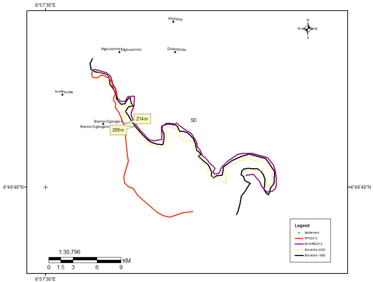
Fig 7: Overlay of 1986 shoreline, 2000, 2013 and RTK at Ogbogoro - Iwofe axis
