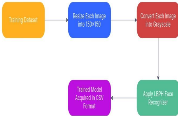
Fig. 3: Training model for face recognition using LBPH face recognition algorithm
