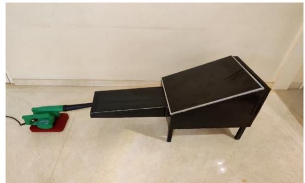
Fig.1: Working Model of Mixed Mode Solar Dryer
