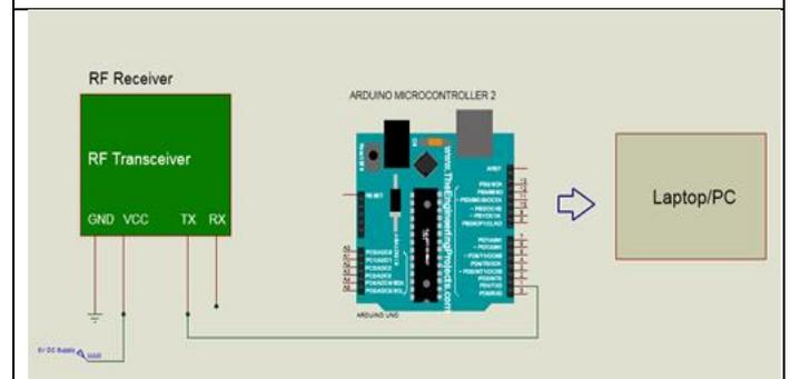
Fig. 2: Schematic diagram of base station.
