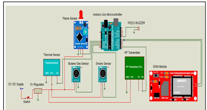
Fig. 1: Schematic diagram of sensor node.
