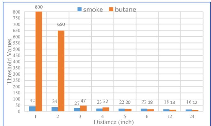
Fig.7: Butane Sensor Test Results
