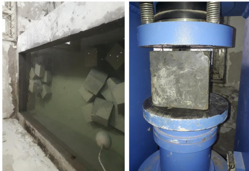
Fig 2: Testing of cube specimen in CTM and curing of concrete cubes
