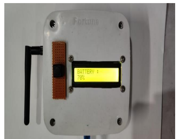
Fig. 17: Battery percentage displayed on LCD
