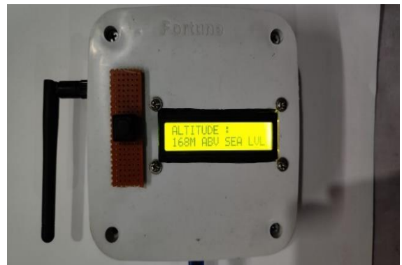
Fig. 16: Altitude displayed on LCD
