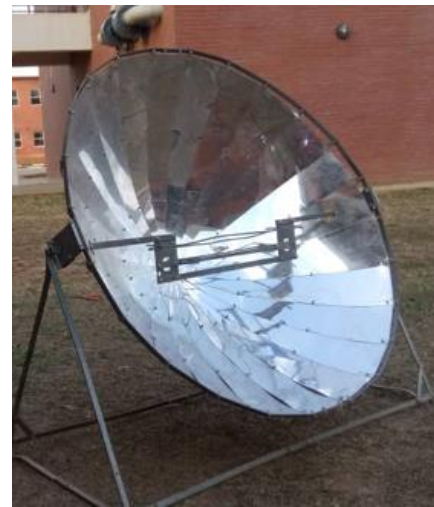
Fig. 3: (a) A schematic of a PDR petal with dimensions and (b) the PDR assembled using all the 24 petals
