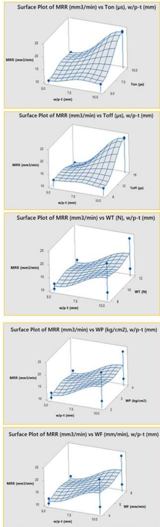
Fig 4.2: Surface Plots of MRR vs.  $w/p-t$  w.r.t Process Parameters
