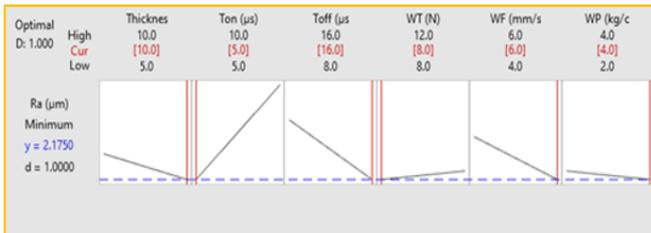
Fig 4.3: Optimization of Ra vs. Process Parameters
