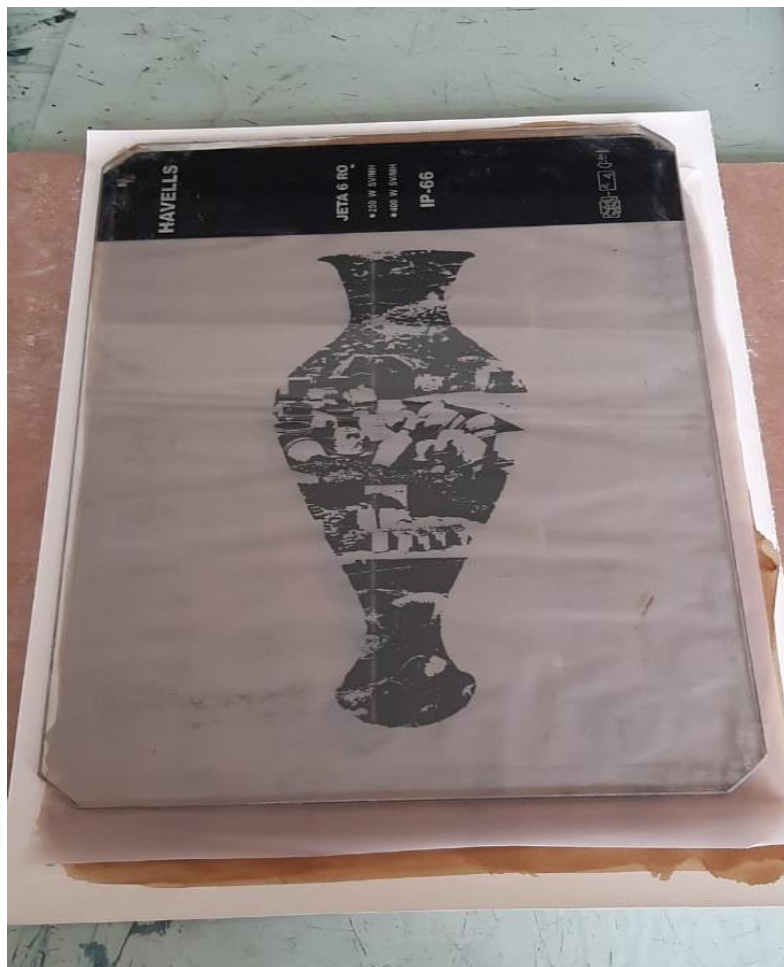
Fig. 21: Place the negative on coated paper then cover it up with the help glass slab for exposure
