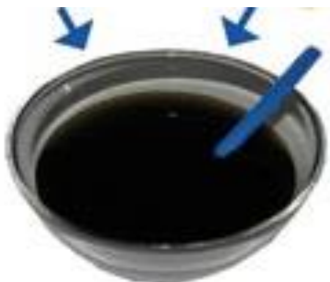
Fig. 18: Coated the paper with mixer of solution A- Potassium ferricyanide B- ferric ammonium citrate
