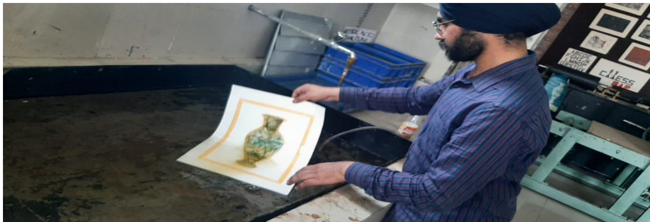
Fig. 22: Add vinegar and water in container with suitable amount. place the exposed print in container for 2 to 5 minutes to remove the extra solution from exposed print.
