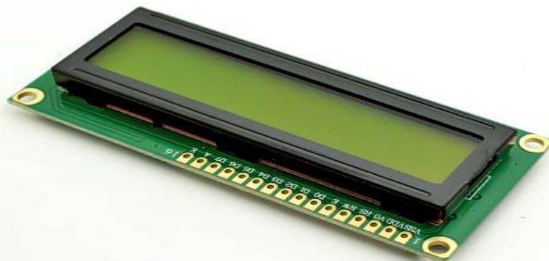
Figure 3.2 Liquid crystal display (16x2 LCD)
