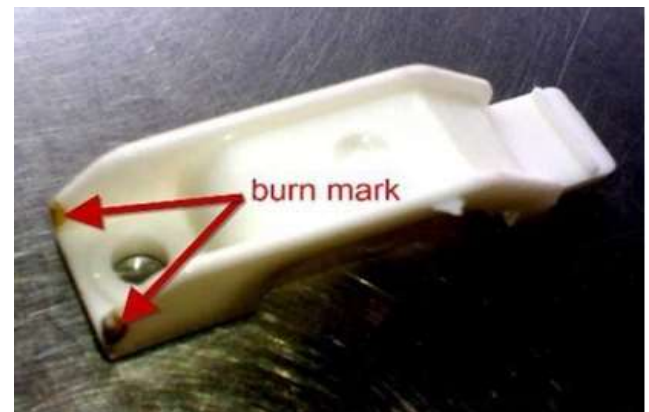
Fig 4.12.5 Burn Marks in component
