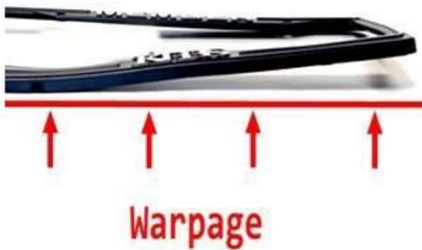
Fig 4.12.7 Warpage in components
