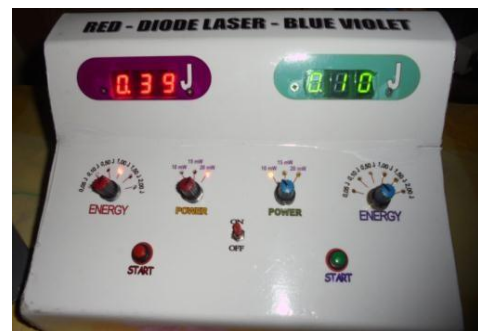
Fig 2. Red and Blue-Violet Diode Laser Control System Display.
