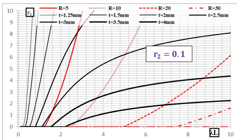
Fig. 10: The suggested values for  $r_1$  for I sections, when applying a direct torque of 0.5 t.cm.
