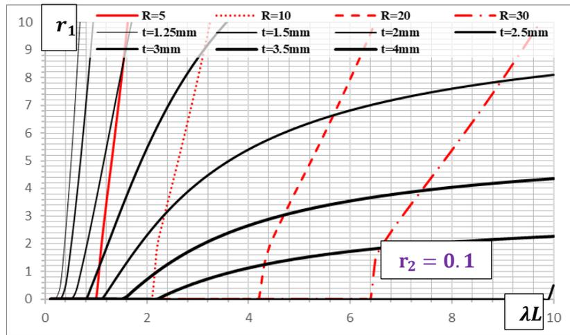
Fig. 7: The suggested values for  $r_1$  for Z sections, when applying a direct torque of 0.5 t.cm
