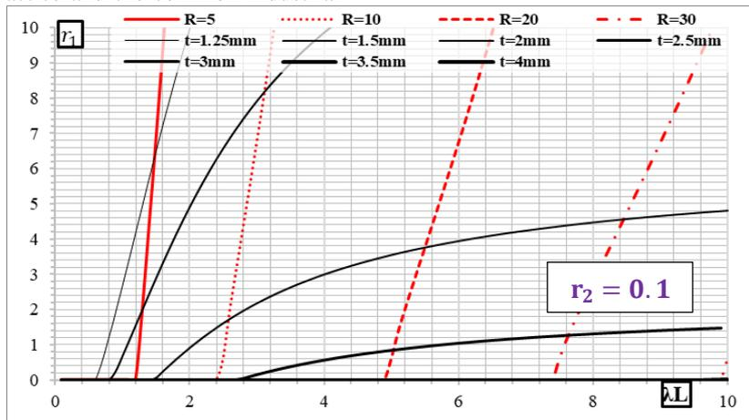
Fig. 3: The suggested values for r<sub>1</sub> for C sections, when applying a direct torque of 0.1 t.cm
