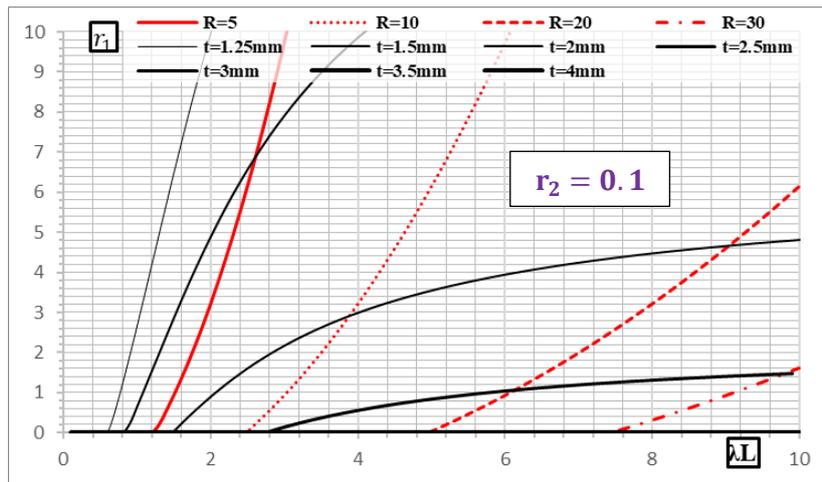
Fig. 9: The suggested values for  $r_1$  for I sections, when applying a direct torque of 0.1 t.cm.
