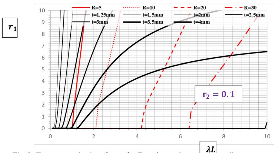
Fig. 8: The suggested values for  $r_1$  for Z sections, when applying a direct torque of 1 t.cm
