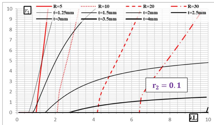
Fig. 6: The suggested values for  $r_1$  for Z sections, when applying a direct torque of 0.1 t.cm
