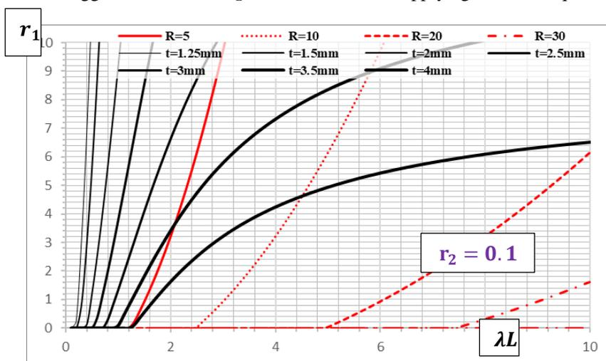
Fig. 11: The suggested values for  $r_1$  for I sections, when applying a direct torque of 1 t.cm.
