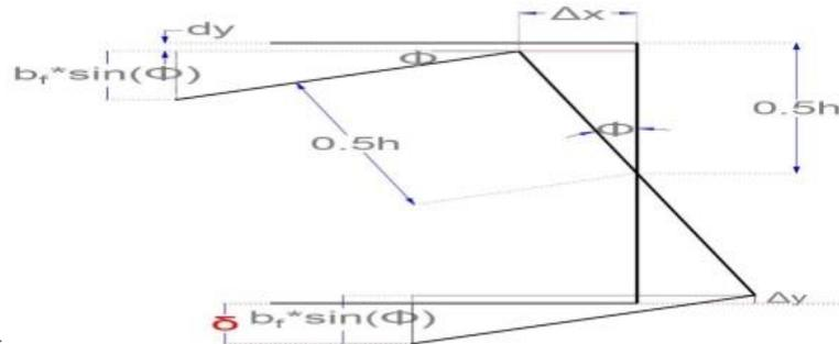
Fig. 2: Relation between the incident twisting angle and the corresponding deflection
