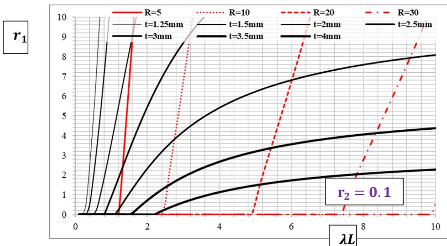
Fig. 4: The suggested values for r<sub>1</sub> for C sections, when applying a direct torque of 0.5 t.cm
