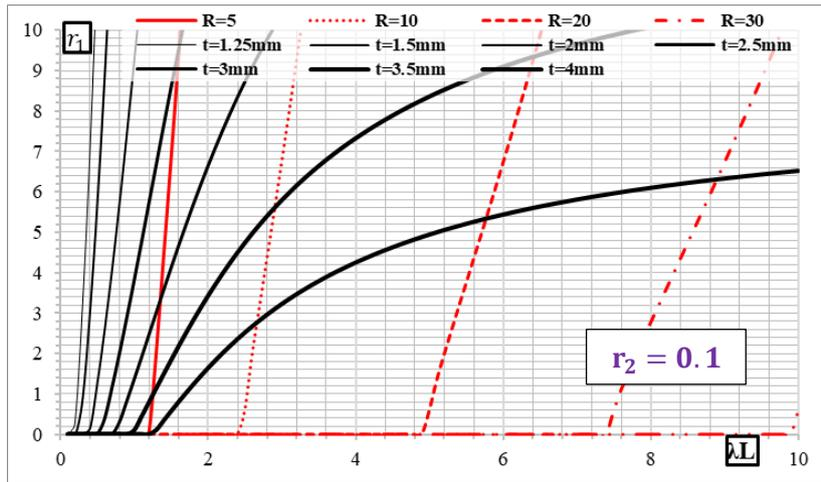
Fig. 5: The suggested values for  $r_1$  for C sections, when applying a direct torque of 1 t.cm
