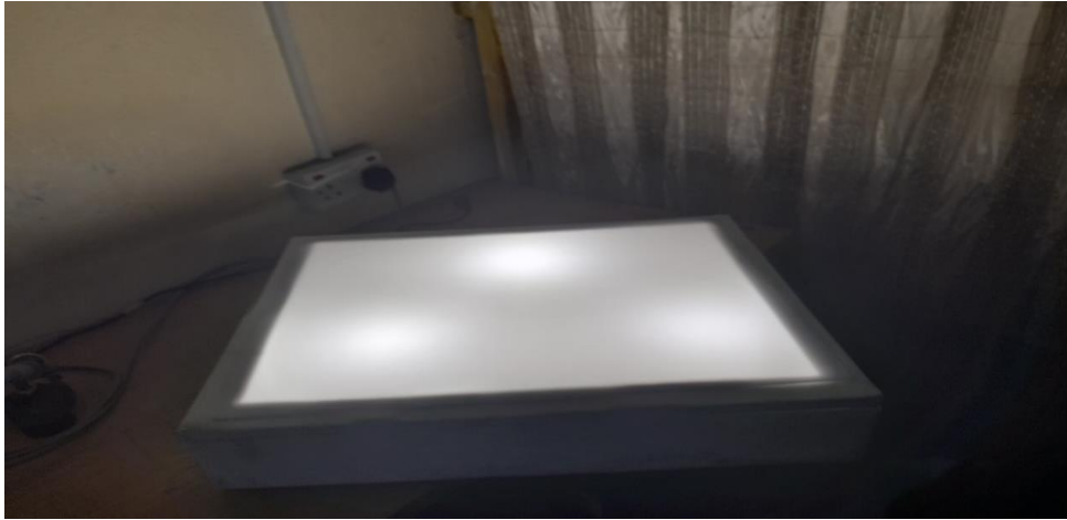
Fig. 3: Fully Powered X-ray viewing box with an alternative power source
