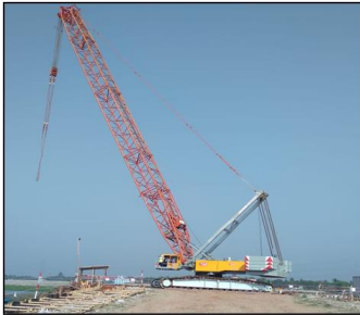
Fig. 3: Lifting Crane for LOLO Jetty Operation
