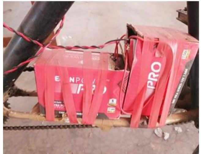
Fig. 10 The 24 V battery pack has been installed in the cycle.
