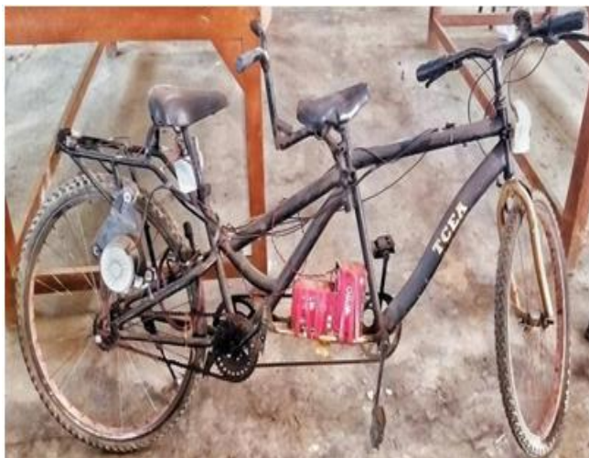
Fig. 5 The electrically driven tandem cycle after installation of motor and auxiliary electrical equipments.
