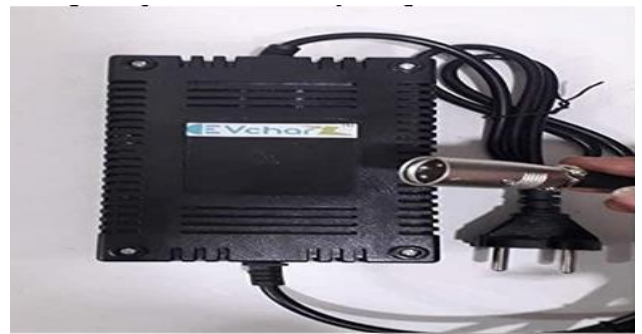
Fig.14 The Battery Charger of 24 V, 4Ah.
