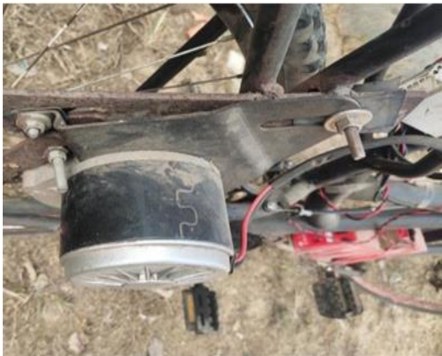
Fig. 9 Permanent Magnet Dc Motor has been installed in the cycle.
