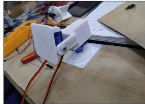
Fig 3.1. 3-D chassis for servo motor
