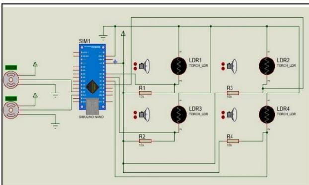
Fig 4.1. Simulation circuit of dual-axis solar tracker
