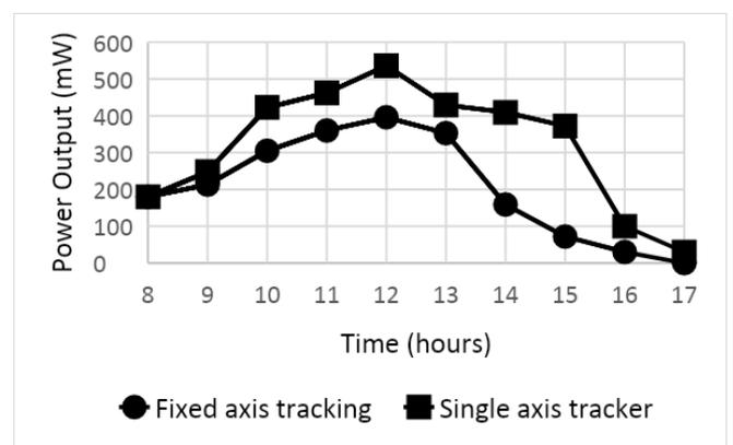
Figure 5.1. Power output from fixed axis tracker Vs. single-axis tracker
