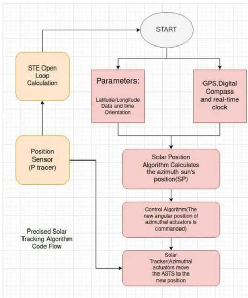
Figure 4.3. Block diagram of precise position algorithm-based controller
