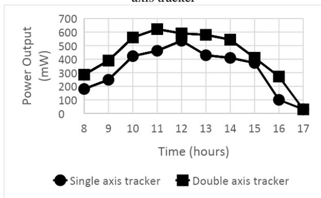
Figure 5.3. Power output from single-axis tracker vs. dual-axis tracker
