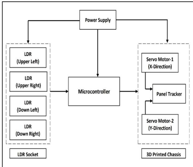
Fig 2.1. Concept behind fabrication of the dual-axis solar tracker
