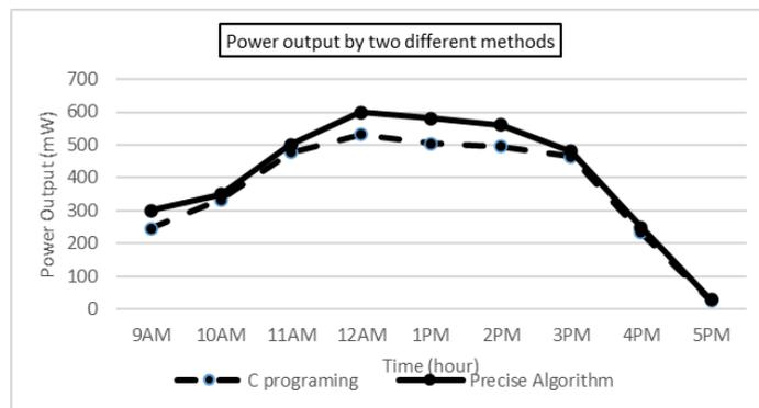
Fig 5.4. Power output as evaluated by C programming and the Precise Position Algorithm
