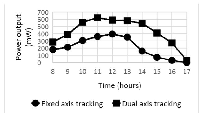
Figure 5.2. Power output from fixed axis tracker Vs. dual-axis tracker
