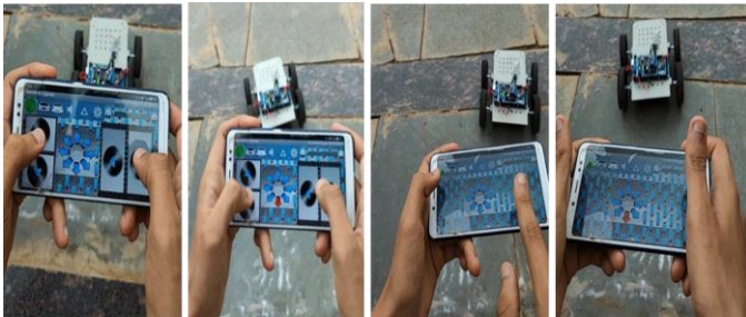
Fig. 8: Robot controlled via Joystick and Gyroscopic sensor.
