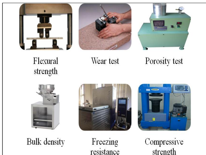
Fig 4 The Tests Conducted for Obtaining the Physical Parameters of the White Carrara Marble
