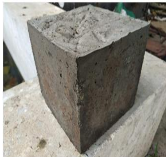
Fig 7 Ash Replaced Concrete Cube
