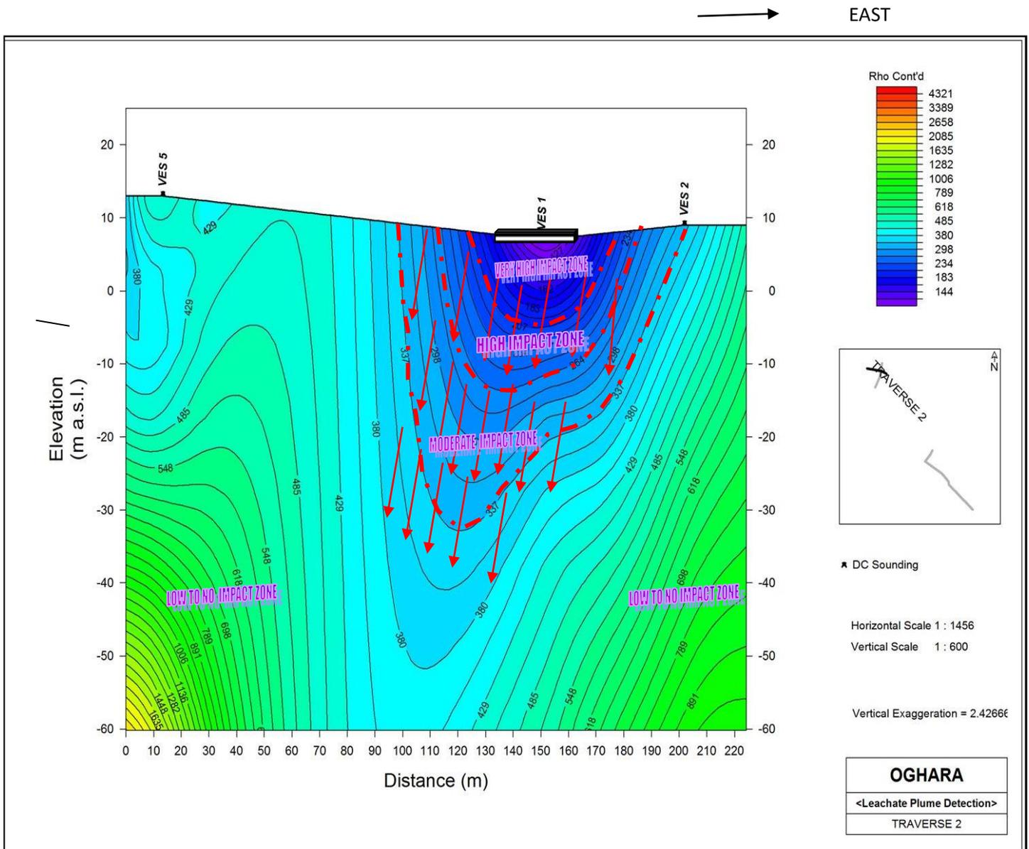
Fig. 7: The 2-D Section Beneath Profile 2
