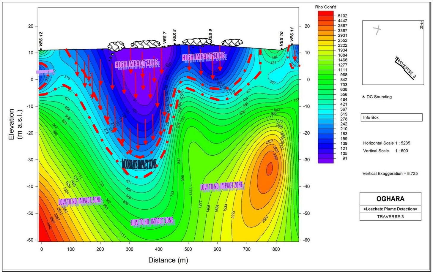
Fig. 8: The 2-D Section Beneath Profile 3
