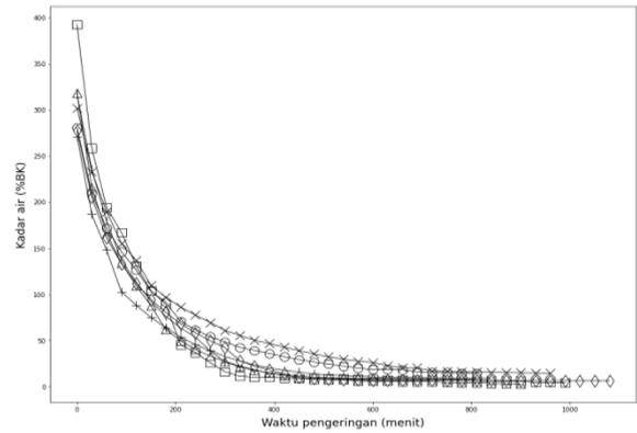
Fig 2:- The moisture content at a drying temperature of 65 °C
