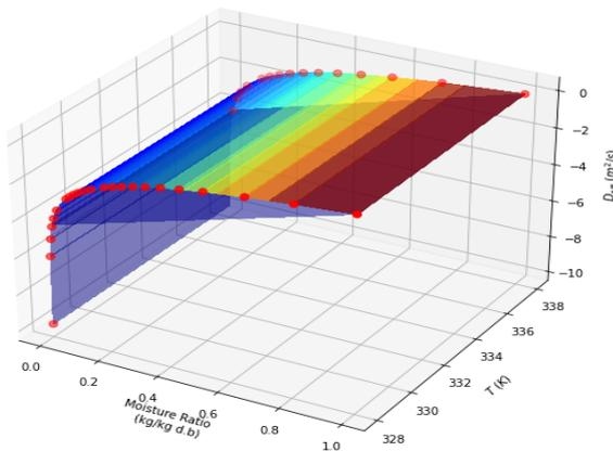
Fig 8:- Experimental simulation of effective moisture diffusivity without blanching
