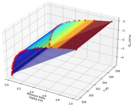
Fig 7:- Experimental simulation of effective moisture diffusivity with blanching
