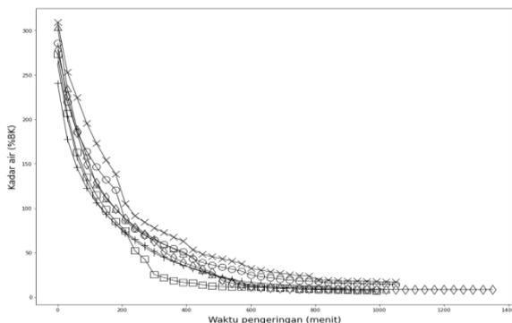
Fig 1:- The moisture content at a drying temperature of 55 °C
