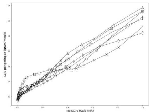
Fig 3:- Drying rate versus humidity ratio at a drying temperature of 55 °C
