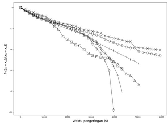
Fig 5:- Effective diffusivity of breadfruit on drying at 55 °C
