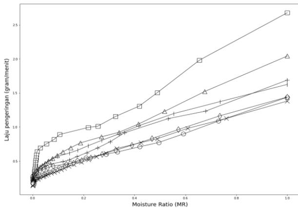
Fig 4:- Drying rate versus humidity ratio at drying temperature of 65 °C
