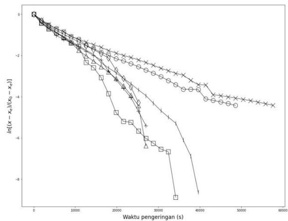
Fig 6:- Effective diffusivity of breadfruit on drying at 65 °C
