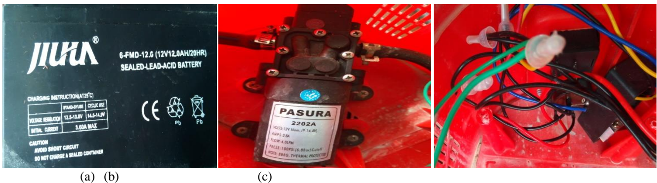
Fig.2: (a) Battery, (b) Pump, (c) Interconnections
