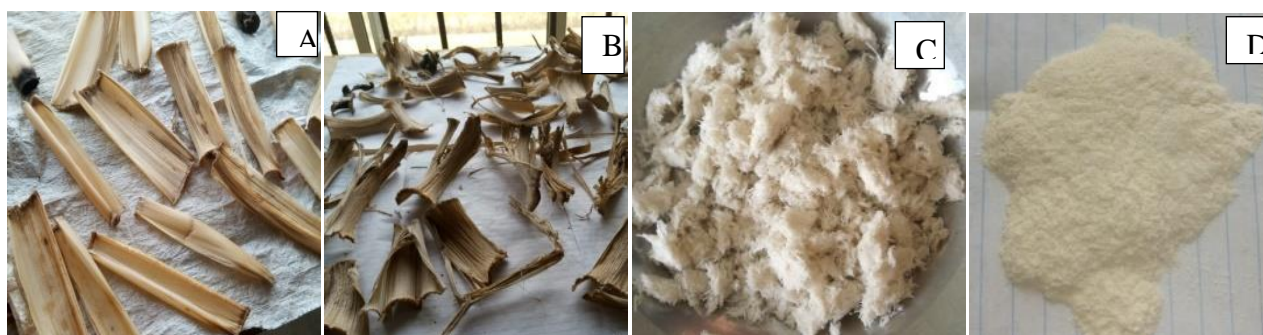
Fig. 1: A- Freshly cut banana pseudostem, B- Dried banana pseudostem, C- Delignified and bleached banana pseudostem and D- Banana pseudostem cellulose powder
