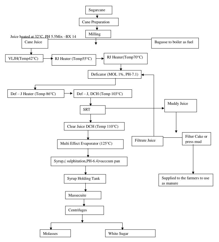
Juice is extracted in the milling plant and heated many times at different degrees of Celsius and also treated by double sulphitation process in this sugar industry. In this double sulphitation process, raw juice which has 5.5PH level is heated at 32°C and passed it to vapour line juice heater to raise its temperature from 32°C to 70°C in different tanks.
