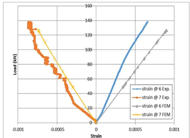
Fig. 20: Comparison of experimental and FEM load-strain curve of interior diagonal webs for Model 2.
