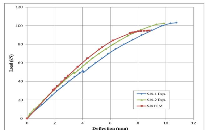
Fig. 13: Comparison of experimental and finite element load-deflection curve for model 1 specimens.
