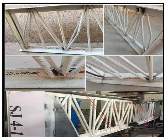
Plate (1): Mode of failures of Model 1 HOWSJ specimens.
