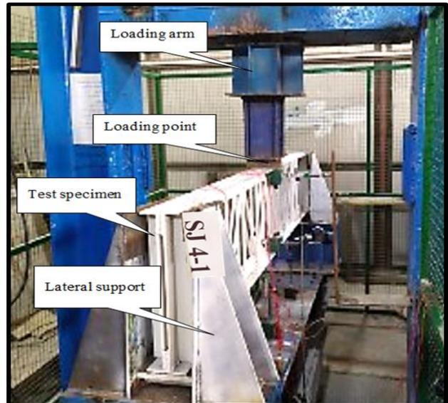
Fig. 2: Details of HOWS Joists Setup.
