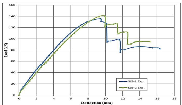
Fig. 4: Experimental load-deflection curve for Model 2 specimens.
