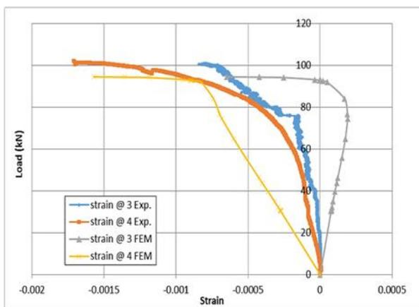
Fig. 16: Comparison of experimental and FEM load-strain curve of top chord for Model 1.
