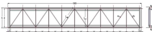
Fig. 1: Prefabricated Hybrid Open Web Steel Joists (all dimensions in mm).
