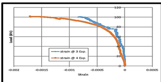
Fig. 7: Load-strain curve of top chord of Model 1 HOWSJ specimens.
