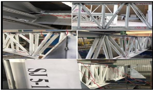
Plate (2): Mode of failures of Model 2 HOWSJ specimens.
