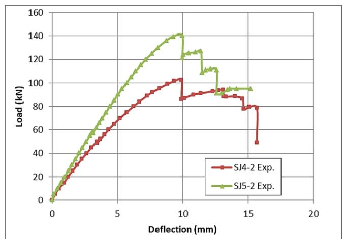
Fig. 5: Load-deflection curve for SJ4-2, and SJ5-2 specimens.
