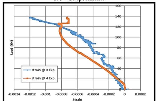
Fig. 10: Load-strain curve of top chord of Model 2 HOWSJ specimens.
