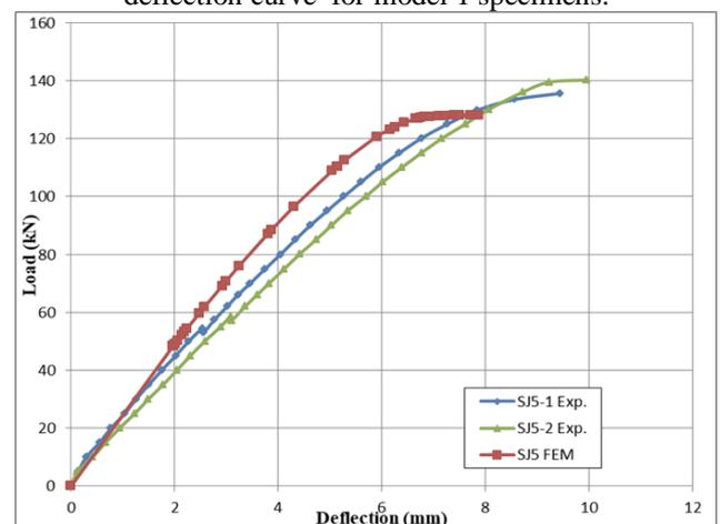
Fig. 14: Comparison of experimental and finite element load-deflection curve for model 2 specimens.
