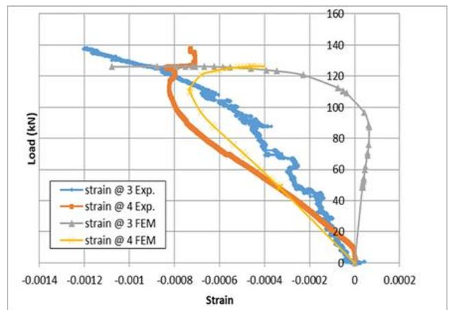
Fig. 19: Comparison of experimental and FEM load-strain curve of top chord for Model 2.
