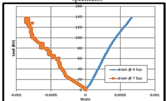
Fig. 11: Load-strain curve of interior diagonal webs near support of Model 2 HOWSJ specimens.
