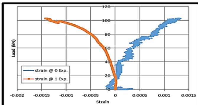
Fig. 6: Load-strain curve of bottom chord of Model 1 HOWSJ specimens.
