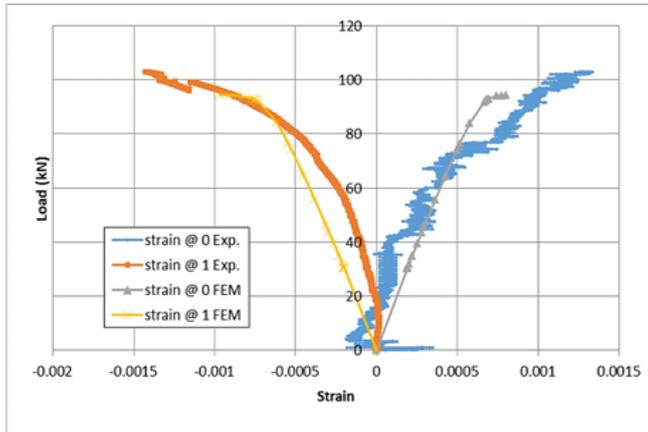
Fig. 15: Comparison of experimental and FEM load-strain curve of bottom chord for Model 1.
