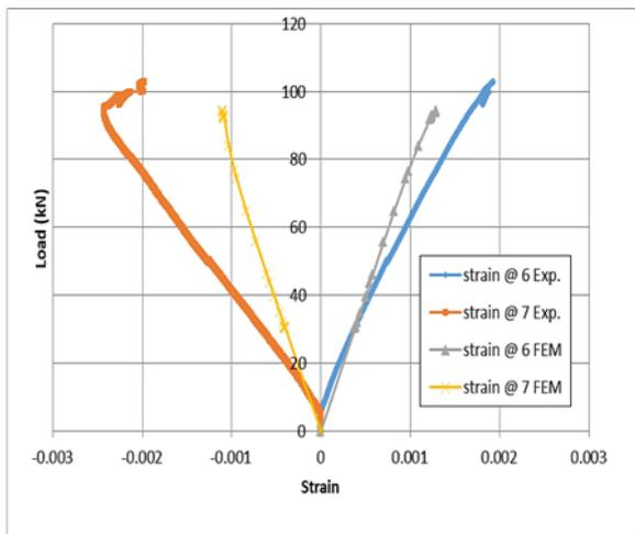
Fig. 17: Comparison of experimental and FEM load-strain curve of interior diagonal webs for Model 1.
