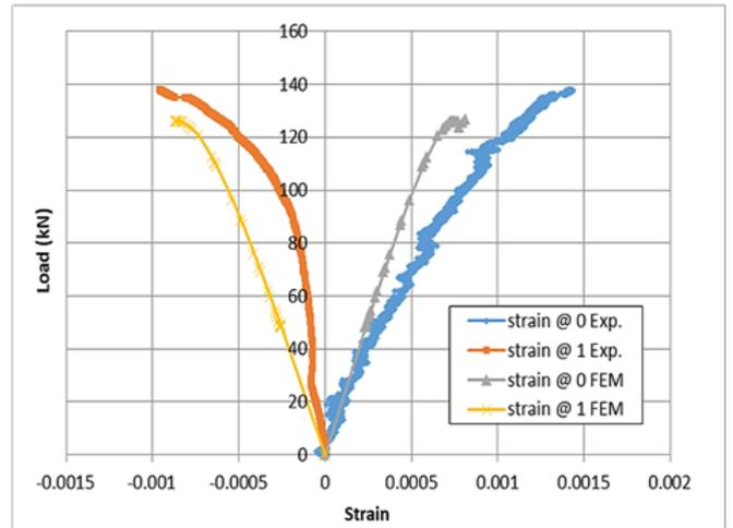
Fig. 18: Comparison of experimental and FEM load-strain curve of bottom chord for Model 2.
