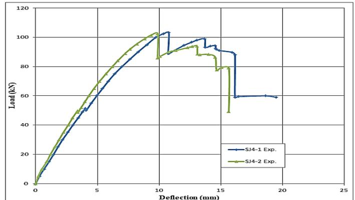
Fig. 3: Experimental load-deflection curve for Model 1 specimens.
