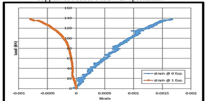
Fig. 9: Load-strain curve of bottom chord of Model 2 HOWSJ specimens.
