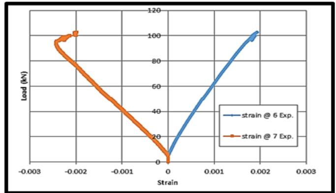
Fig. 8: Load-strain curve of interior diagonal webs near support of Model 1 HOWSJ specimens.
