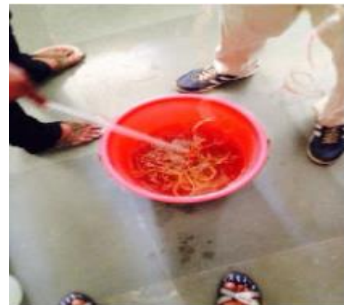
Fig 5: Soaking of fiber in NaOH solution
