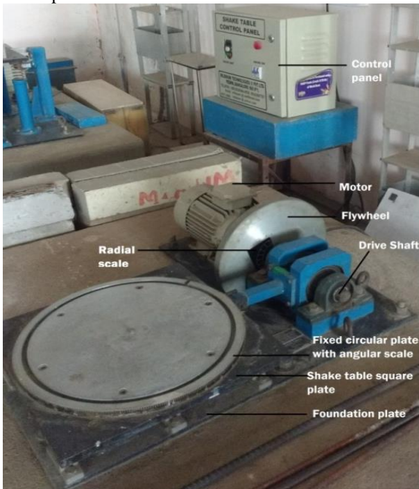
FIGURE 3.2: SHAKE TABLE WITH CONTROL UNIT
