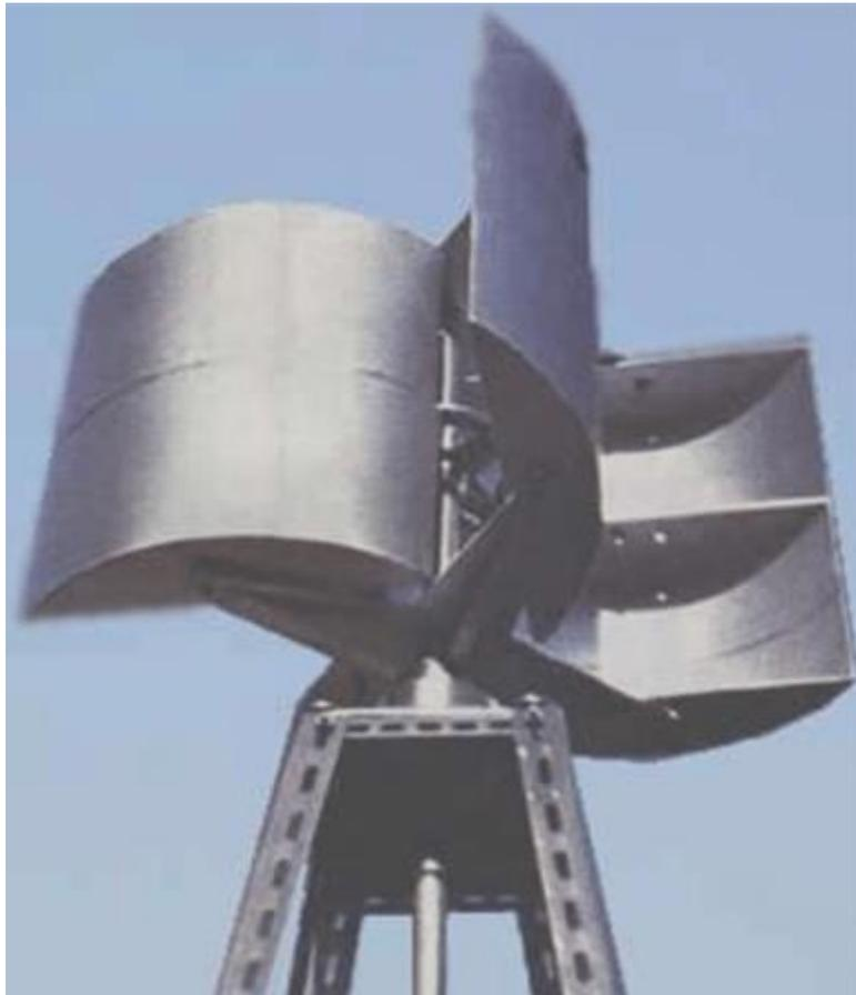
Fig 1.4: Simple Savonius Wind Turbine – 3 Blades.
