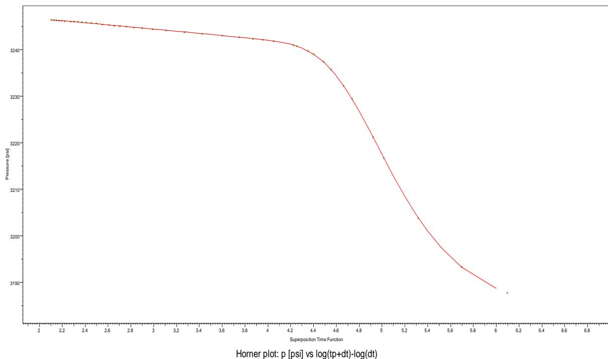
Fig 8: The Horner plot [Semilog plot of bottom-hole pressure vs  $\log (tp + \Delta t) / \Delta t$ ]
