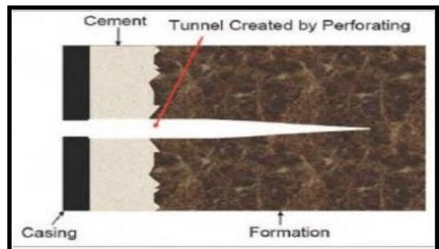
Fig 2: The perforation process (Source: Halliburton 2012, cited in, Elmouzemill, 2017).
