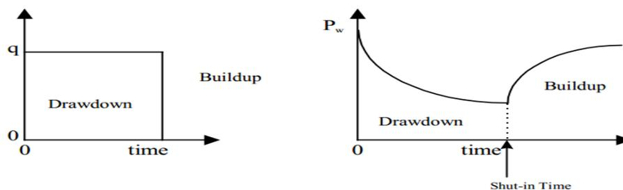
Figure 3: Rate and Pressure Profiles During Drawdown and Build-up (Source: Onyekonwu, 1997)
