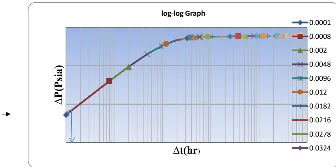
Fig 11: Excel sheet Showing the Log-Log Plot for the Buidup test analysis
