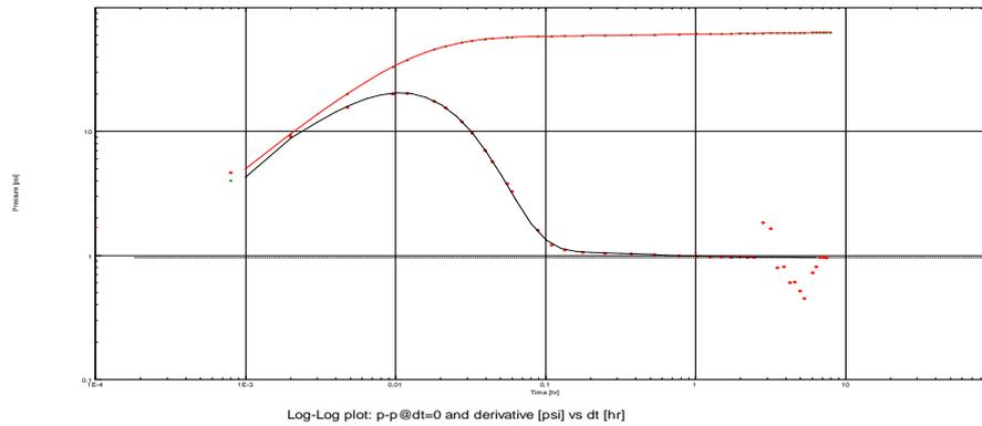
Fig 9: Log-Log plot of differential pressure(dp) and pressure derivative(dp') vs.dt(hr)
