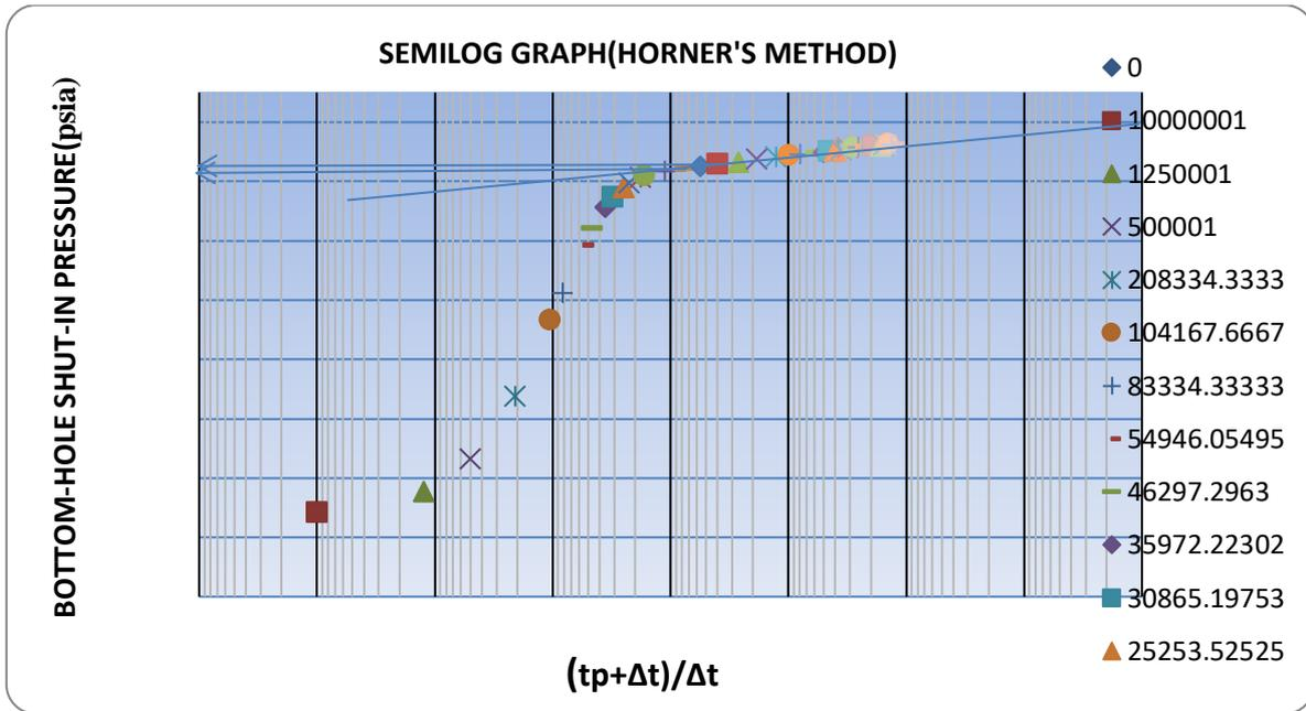
Fig 12: Excel Sheet Showing the Semilog Plot for the Build-up test analysis.
