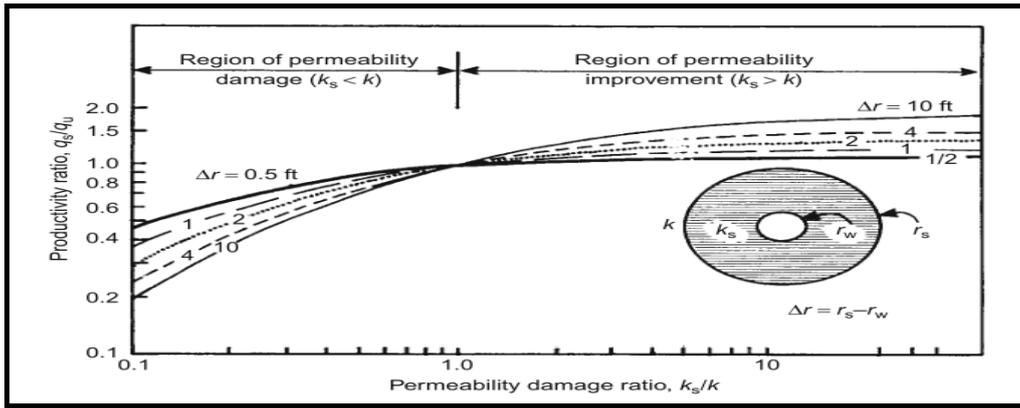
Fig 1: The effect of permeability damage on wells productivity ratio (Source:Tiab & Donaldson,2004).
