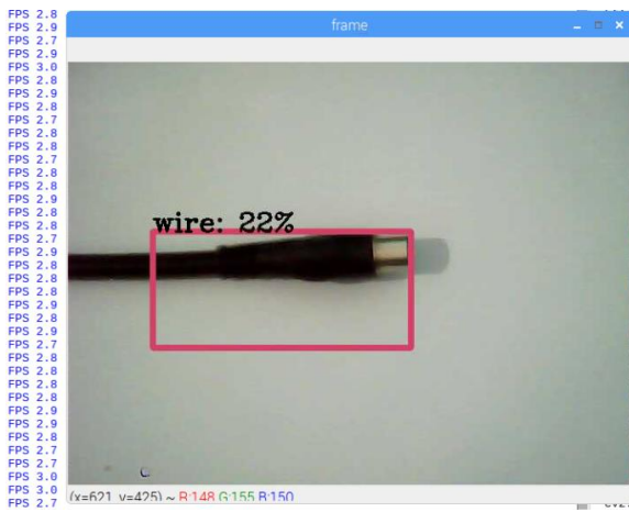
Figure 2 : Architecture 1 Result for TV Antenna Cable End Detection on Raspberry Pi 3B+
