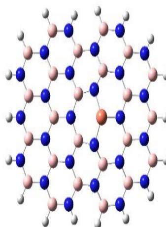
Fig. 2: represent geometrical structure of BN-Cu nano-ribbon.
